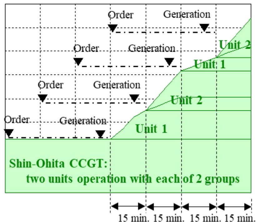
Figure 6. Generation Units Operation during a ramp-up in the evening on April 30th.
