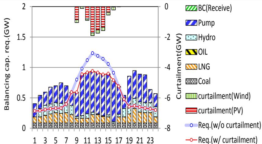
Example: LFC capability balance and generation curtailment
